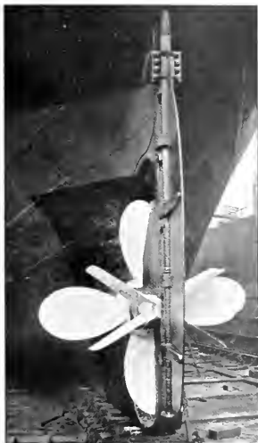
View of stern of the steamship Norfolk on the dock at the Robins Plant, showing contrapropeller in place as installed by Todd Shipyards Corporation.
